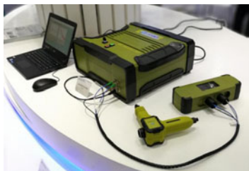
Fig. 8 Main components to the fiber coupled time-domain spectrometer in operation
