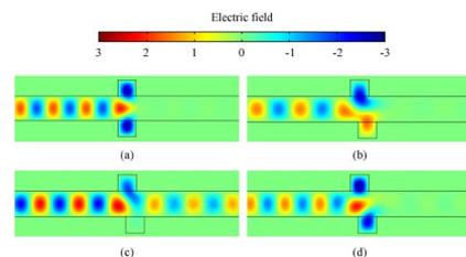
Fig. 4. Electric field distribution of PPWG-cavities systems inside the waveguide at the resonant and transparency peak frequencies with  $S = 650$   $\mu\text{m}$ : (a)  $L = 0$   $\mu\text{m}$  at 0.419 THz, (b)  $L = 200$   $\mu\text{m}$  at 0.359 THz (the lower frequency resonance dip), (c)  $L = 200$   $\mu\text{m}$  at 0.383 THz (the transparency peak), and (d)  $L = 200$   $\mu\text{m}$  at 0.41 THz (the higher frequency resonance dip).
