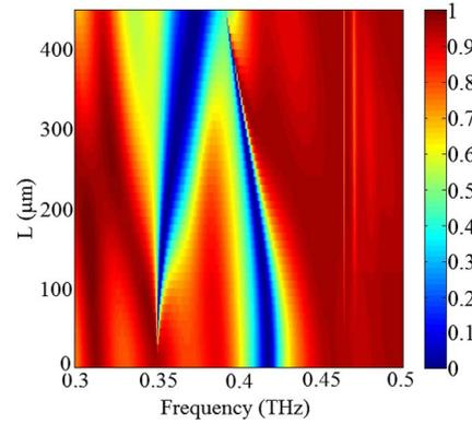
Fig. 3. Simulated transmission amplitude of PPWG-cavities systems as a function of the asymmetric shifting length  $L$ .
