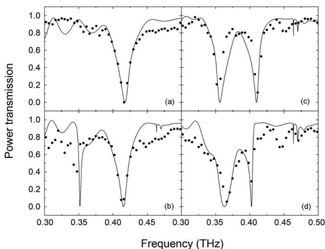
Fig. 2. Power transmission spectra for (a)  $L = 0$   $\mu\text{m}$ , (b)  $L = 100$   $\mu\text{m}$ , (c)  $L = 200$   $\mu\text{m}$ , and (d)  $L = 300$   $\mu\text{m}$ . The solid lines are the numerical results based on the finite element method. The dots represent the power transmission spectra (the frequency resolution  $\sim 4.58$  GHz) derived by Fourier-transforming the 218.4 ps time-domain waveforms and compared to a PPWG without cavities.
