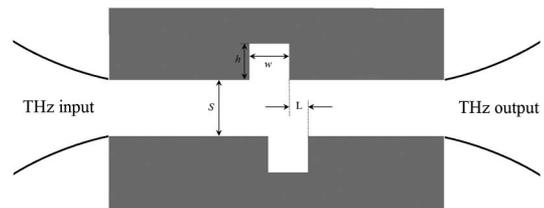
Fig. 1. Schematic of PPWG with two cavities.  $w$ , the width of the groove;  $h$ , the depth of the groove;  $S$ , the length of the plates;  $L$ , the shifting length between two grooves.
