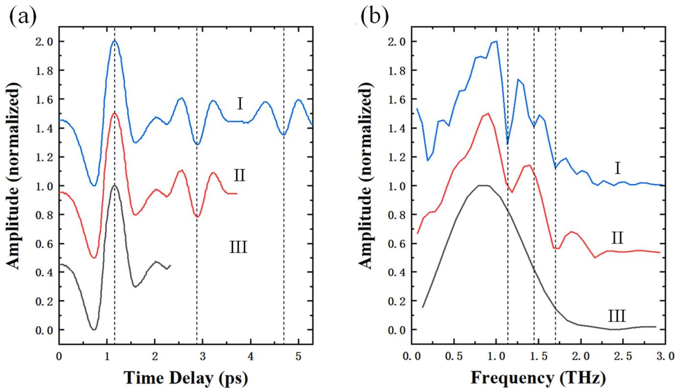
**Figure 5.** THz signals with water absorption in the (a) time and (b) frequency domain, with different temporal widths or spectral resolutions. Vertical lines in (b) mark the three spectral dips of the top signal. Data of (a-I) is from Ref. [20].
