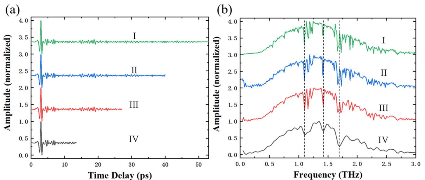
**Figure 4.** THz signals with the water absorption in the (a) time and (b) frequency domain, with different temporal widths or spectral resolutions. The vertical lines in (b) marked the same spectral dips of all the signals. Data of (I) in (a) is from Ref. [21].
