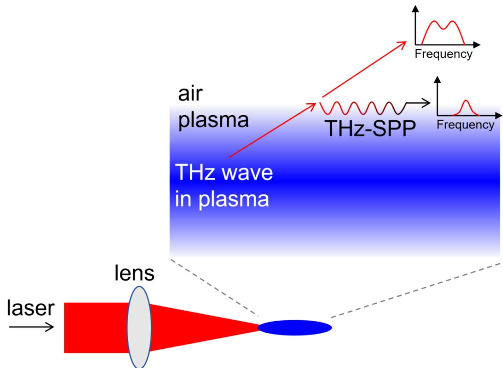
**Figure 6.** A schematic diagram of THz-SPW generation in the region of a plasma filament column.
