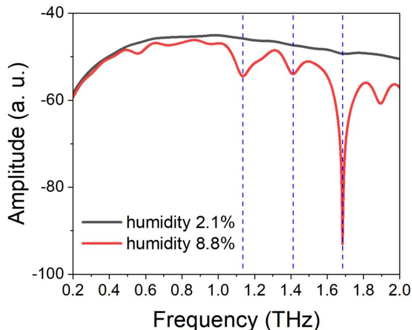
**Figure 3.** The THz spectra emitted from a two-color laser filament under two humidity values of air.
