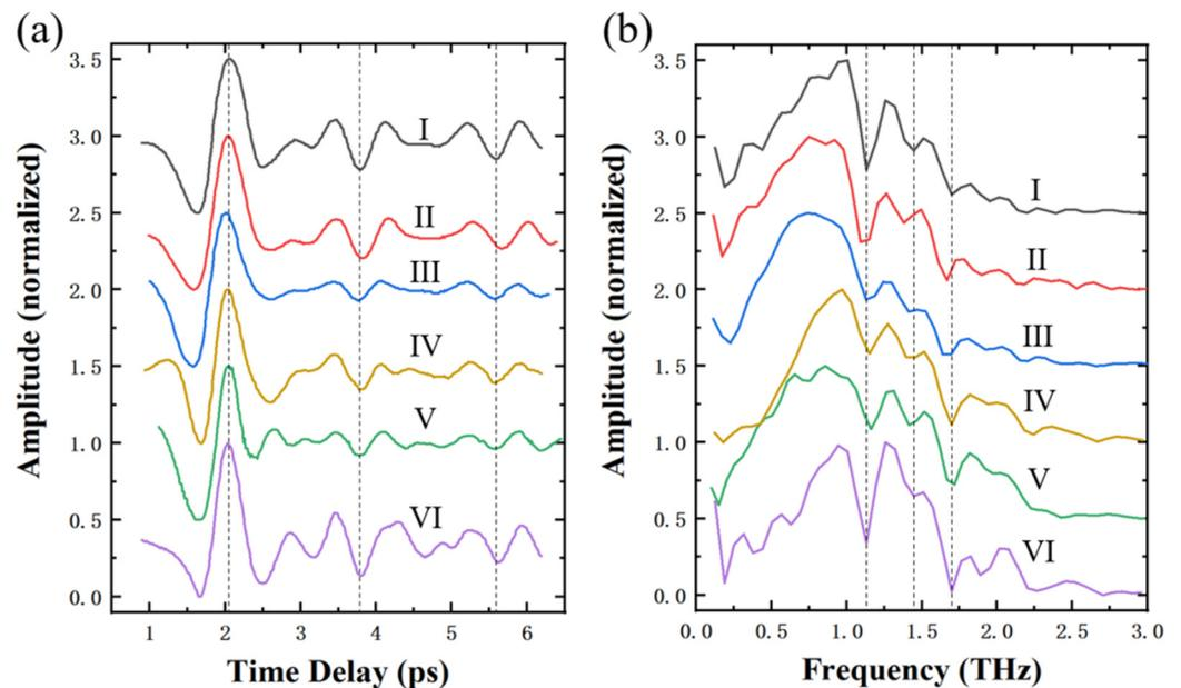
**Figure 2.** THz signals extracted from the literature [18,20–24] for the (a) time and (b) frequency domain, respectively. Vertical lines mark the same peaks or valleys of all the signals. Four signals of (I–IV) are from laser-filament-based THz sources, while the other two (V, VI) are from nonlinear-crystal-based THz sources.
