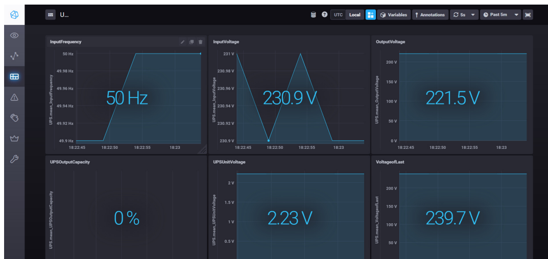
Figure 1. Example of the custom dashboard. The dashboard displays the time curve and current value of parameters of the UPS, such as the input voltage and the frequency.
