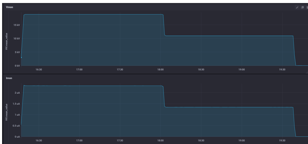
Figure 6. Example of the voltage (top) and current (bottom) from the Matsusada AU HV power supplies during a data taking run, collected by the P-SCS.
