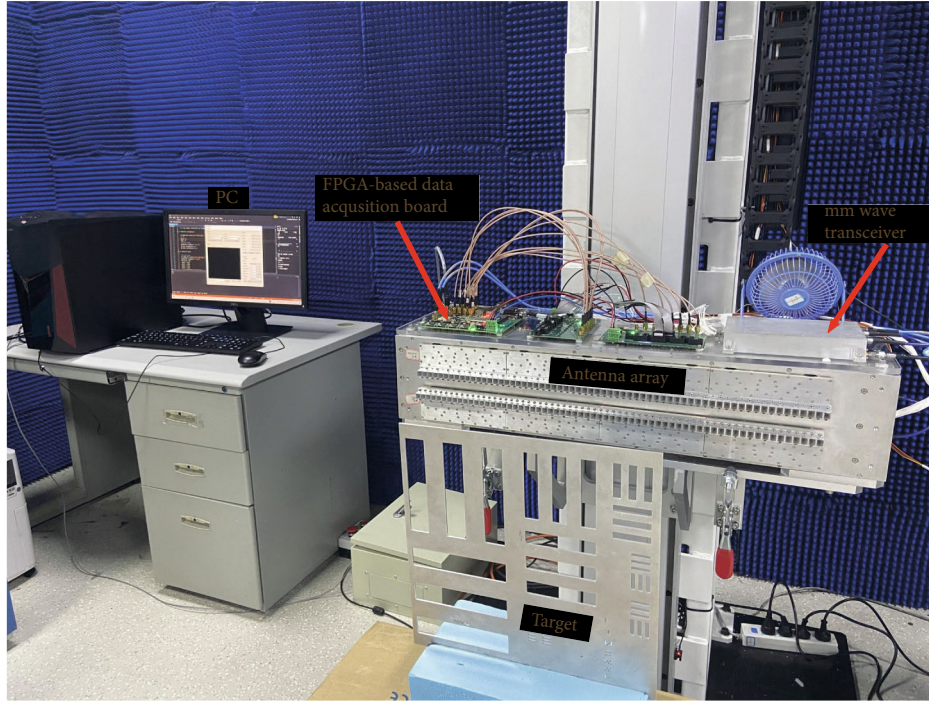
FIGURE 5: The setup of the 3D mmWave radar imaging system.
